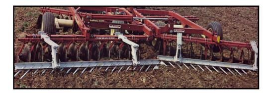
The Precision Buster Bar harrow attachment is designed to attach to secondary tillage tools such as disks or cultivators. By disking and harrowing in one trip, you save time and fuel and do a better job of working up your ground. This improves the seedbed by conserving moisture and prepares the soil for better incorporation of chemicals.
