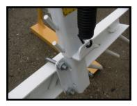
Vertical height adjustment with pin lets you match buster bar to the implement. Suspension spring suspends harrow bar while in transport.
