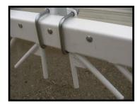
Double u-bolt mounting securely mounts tooth bar to each carrying arm. Clean smooth bar clears trash and avoids dirt build up. Heavy duty 7/8"x9 1/2" bolt on teeth give good penetration and long life. Vertical center teeth prevent ridging.
